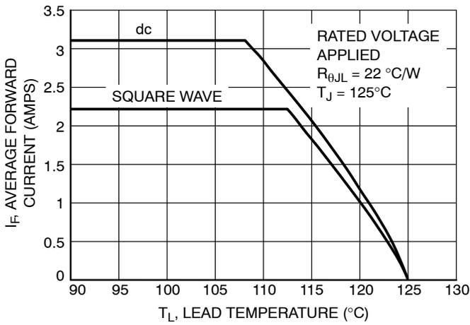
**Figure 4. Current Derating – Junction to Lead**
