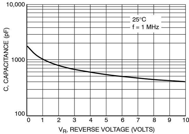
**Figure 6. Typical Capacitance**
