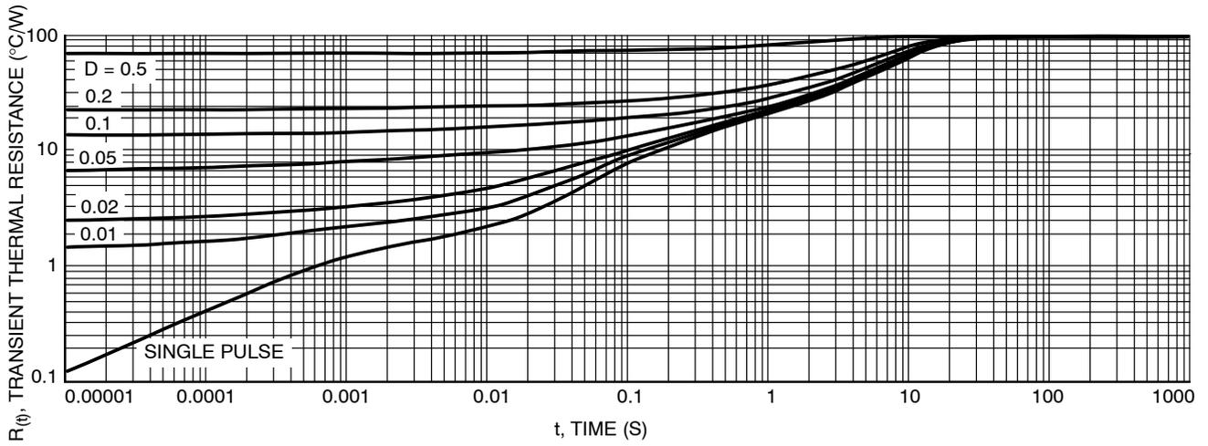
Figure 7. Thermal Response, Junction to Ambient (min pad)
