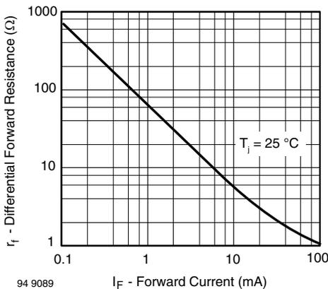
Fig. 3 - Differential Forward Resistance vs. Forward Current
