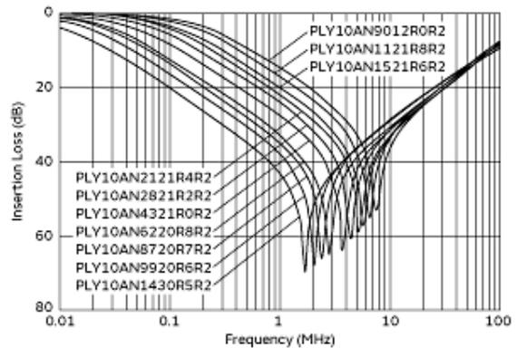
Differential Mode Insertion Loss-Frequency Characteristics
