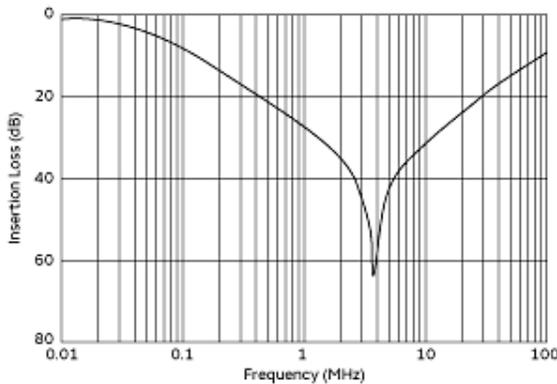
Differential Mode Insertion Loss (Typ.)
