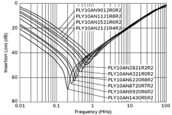
Common Mode Insertion Loss-Frequency Characteristics
