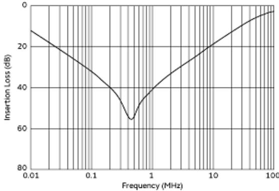
Common Mode Insertion Loss (Typ.)
