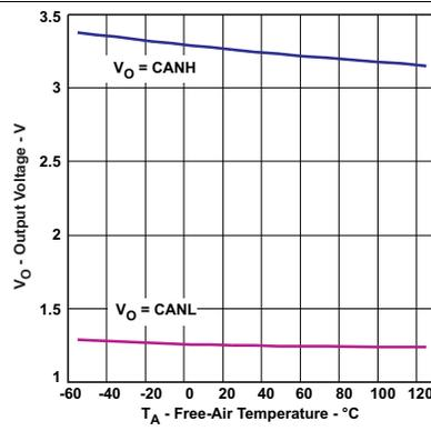
Figure 4. Driver Output Voltage vs Free-Air Temperature
