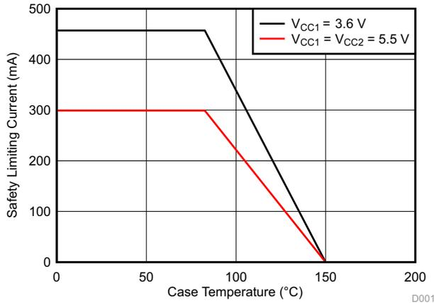
**Figure 21. DUB-8  $\theta_{JC}$  Thermal Derating Curve per VDE**
