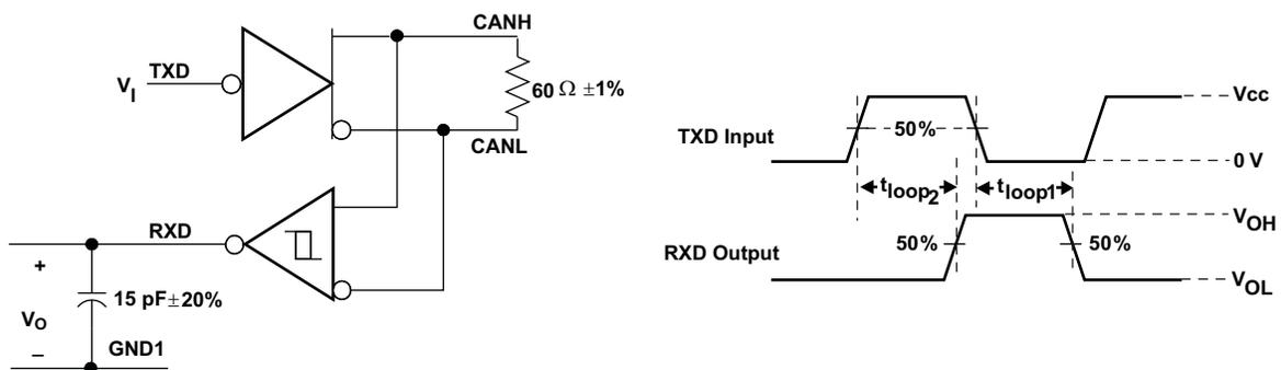
Figure 15.  $t_{\text{LOOP}}$  Test Circuit and Voltage Waveforms
