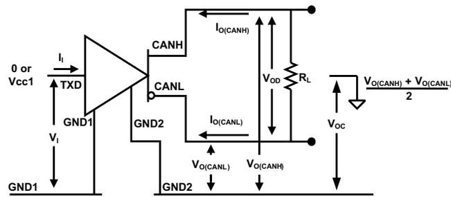
Figure 7. Driver Voltage, Current and Test Definitions
