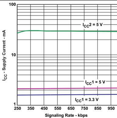
Figure 3. Supply Current (RMS) vs Signaling Rate (kbps)
