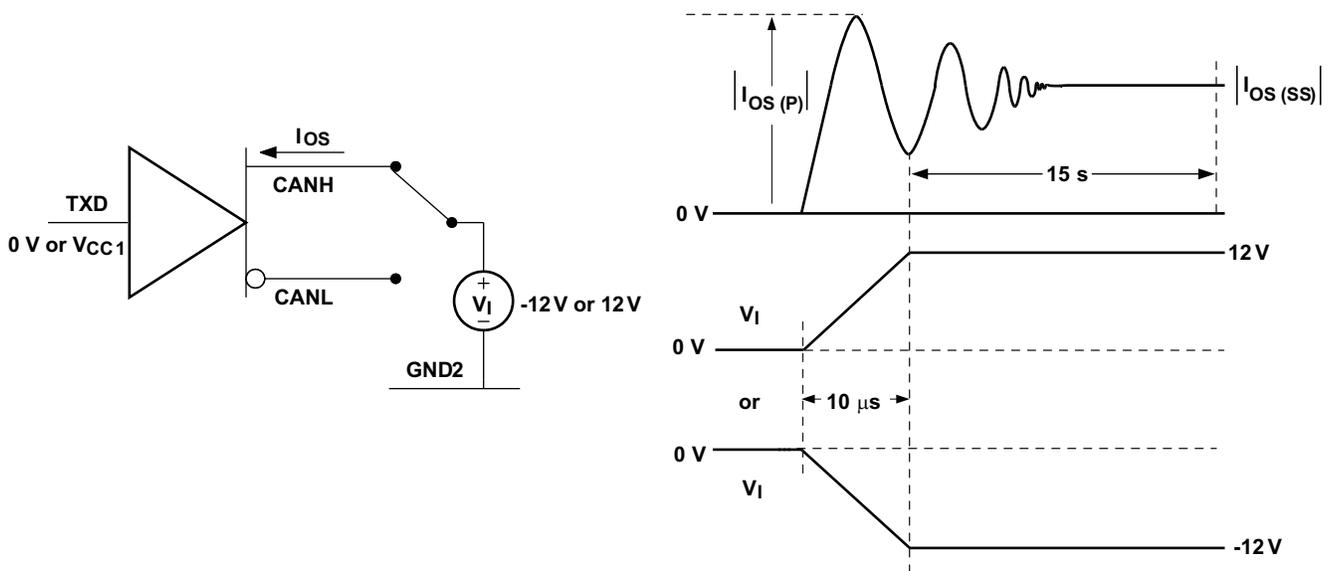
Figure 17. Driver Short-Circuit Current Test Circuit and Waveforms
