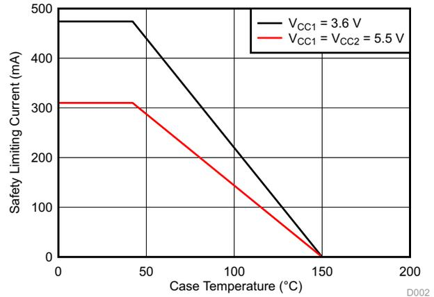
**Figure 22. DW-16  $\theta_{JC}$  Thermal Derating Curve per VDE**
