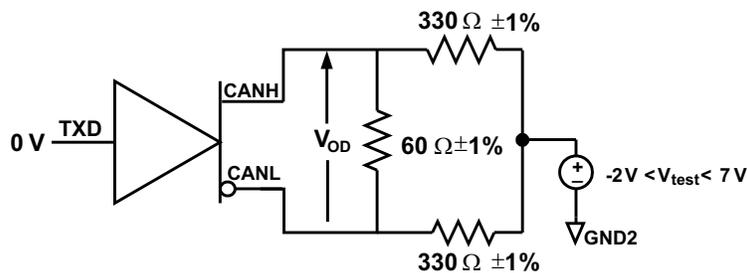
Figure 9. Driver  $V_{OD}$  With Common-Mode Loading Test Circuit
