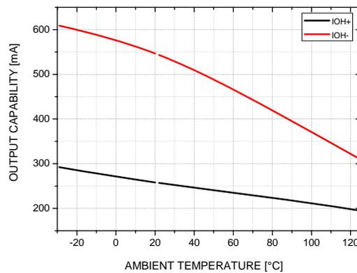
Figure 6. Output Sinking/Sourcing Current vs. Temp.
