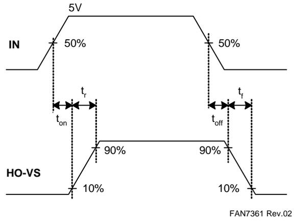
Figure 8. Input / Output Timing Diagram
