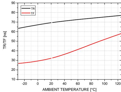
Figure 5. Rising/Falling Time vs. Temp.
