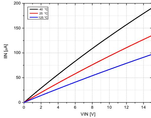
Figure 2. Input Bias Current vs. Input Voltage
