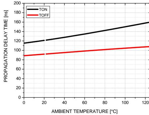
Figure 4. Turn On/Off Propagation Time vs. Temp.
