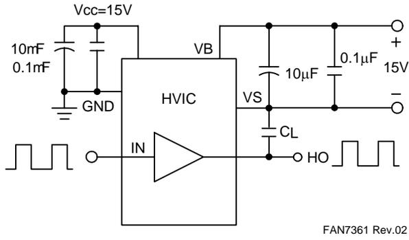
Figure 7. Switching Time Test Circuit
