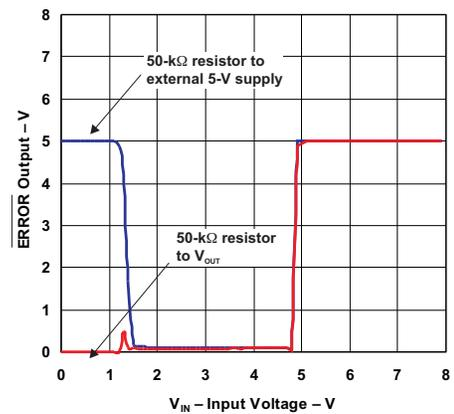
Figure 16. LP2951  $\overline{\text{ERROR}}$  Comparator Output vs Input Voltage
