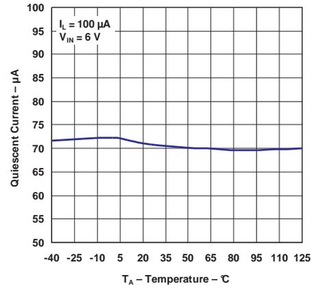
Figure 10. Quiescent Current vs Temperature ( $I_L = 100 \text{ µA}$ )
