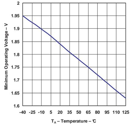
Figure 14. LP2951 Minimum Operating Voltage vs Temperature
