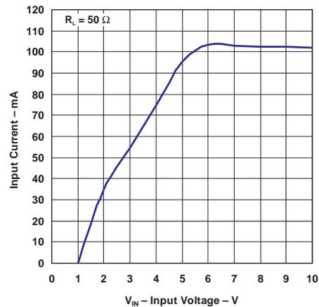
Figure 4. Input Current vs Input Voltage ( $R_L = 50 \Omega$ )
