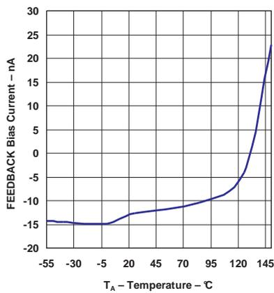
Figure 15. LP2951 FEEDBACK Bias Current vs Temperature
