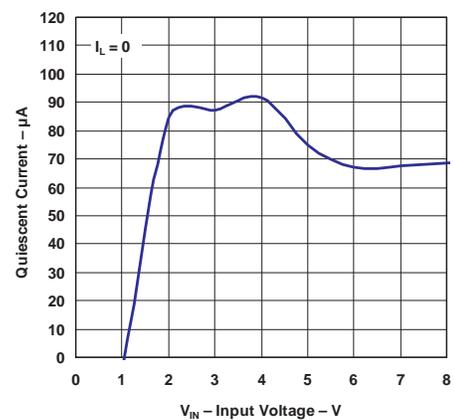
Figure 6. Quiescent Current vs Input Voltage ( $I_L = 0$ )
