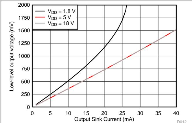
Figure 12. Output Voltage Low ( $V_{OL}$ ) vs Output Sink Current ( $85^\circ\text{C}$ )
