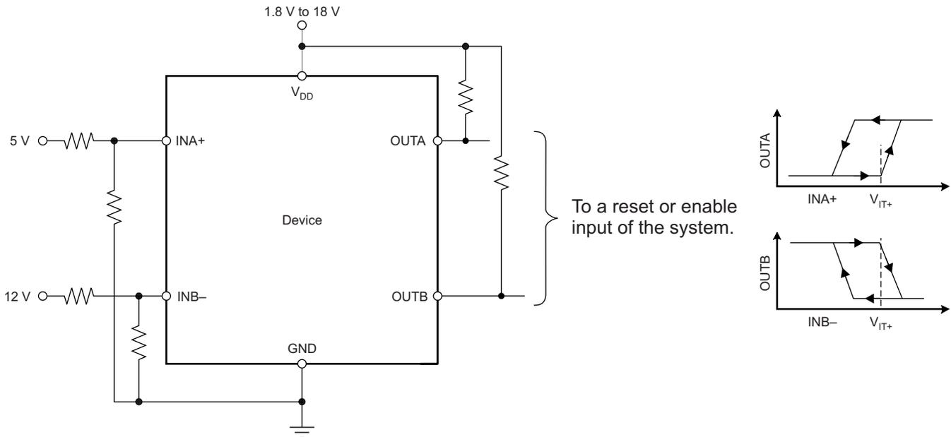
NOTE: In this case, OUTA is driven low when an undervoltage condition is detected at the 5-V rail and OUTB is driven low when an overvoltage condition is detected at the 12-V rail.
