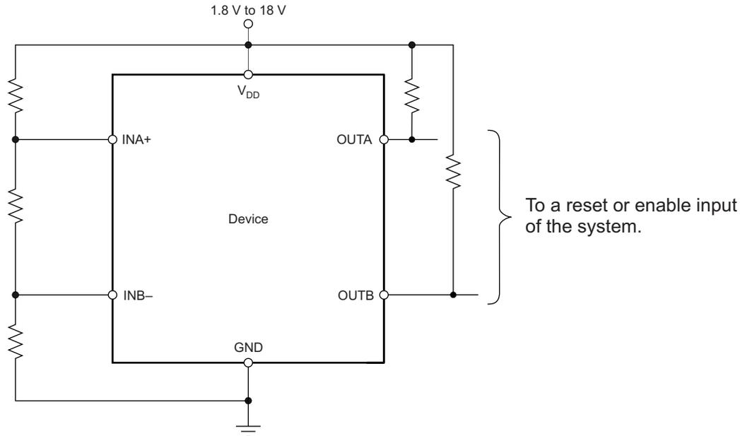
**Figure 17. Monitoring the Same Voltage as  $V_{DD}$**
