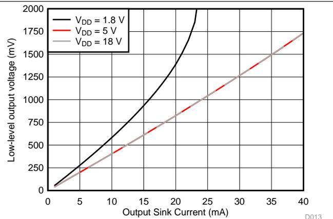
Figure 13. Output Voltage Low ( $V_{OL}$ ) vs Output Sink Current ( $125^\circ\text{C}$ )
