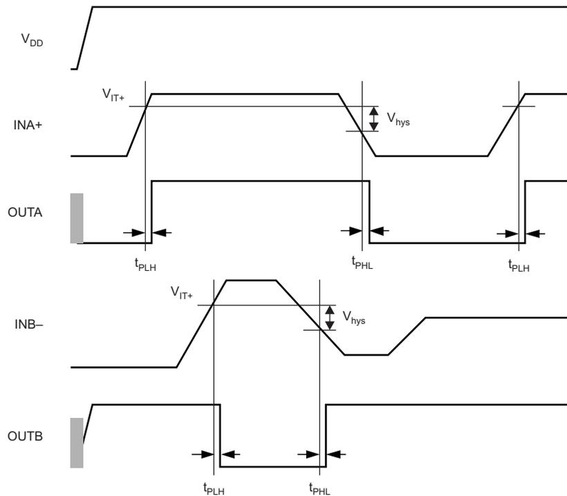
**Figure 1. Timing Diagram**
