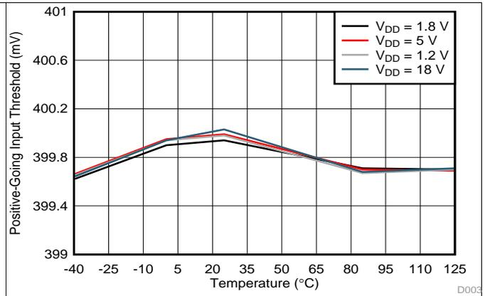
Figure 3. Rising Input Threshold Voltage ( $V_{IT+}$ ) vs Temperature
