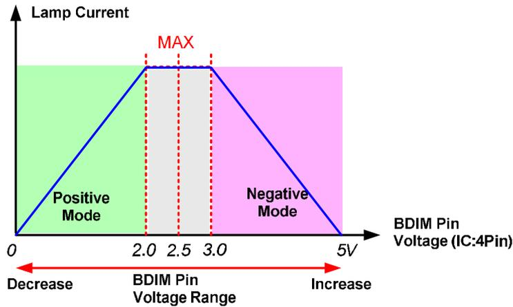
Burst PWM is generated using BDIM and triangular wave of CTB. The rising and falling slopes of BDIM operation are adjusted by capacitor which is connected between ICMP pin and GND. The source and sink currents of ICMP are 100uA. We recommend 300usec as rising and falling time.
