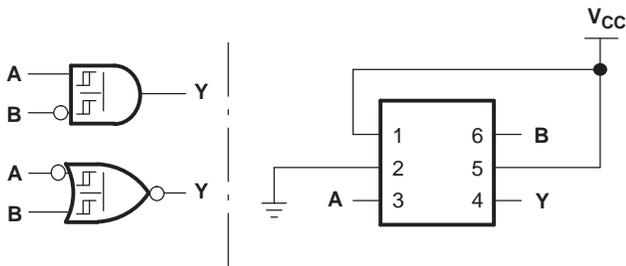
Figure 3. 2-Input AND Gate With Inverted B Input
