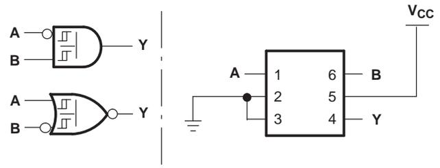
Figure 2. 2-Input AND Gate With Inverted A Input
