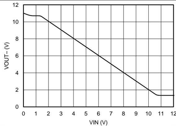
**Figure 7. Positive Output Voltage Node vs Input Voltage**
