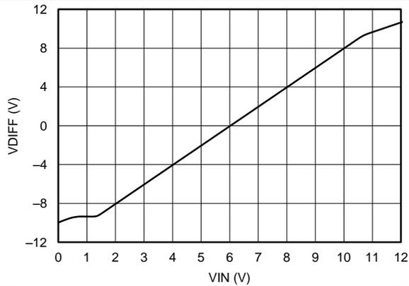
**Figure 5. Differential Output Voltage vs Input Voltage**
