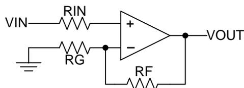
**Figure 8. Operational Amplifier Schematic for Noninverting Configuration**
