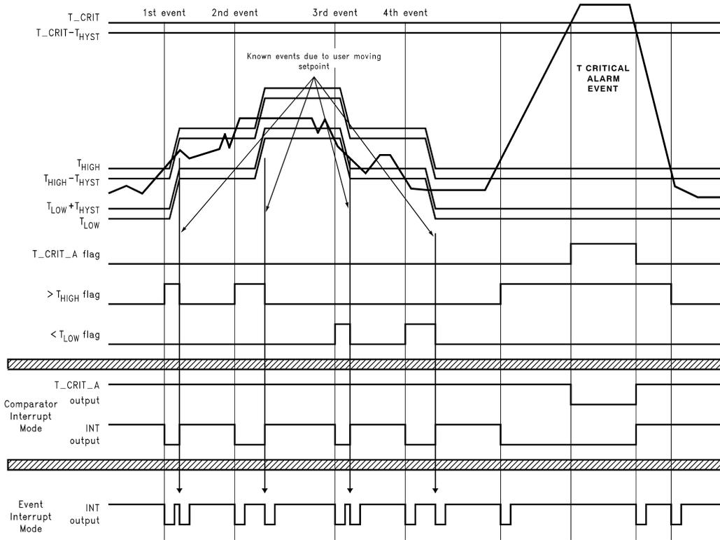
**Note:** Event Interrupt mode is drawn as if the user is reading the part. If the user doesn't read, the outputs would go low and stay that way until the LM77 is read.
