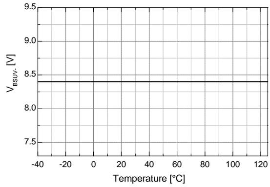
Figure 21. V<sub>BS</sub> UVLO- vs. Temperature
