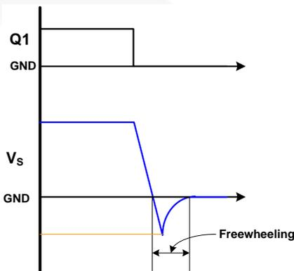
**Figure 35.  $V_S$  Waveforms During Q1 Turn-Off**
