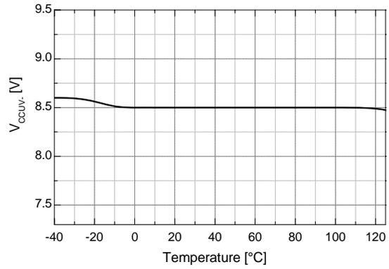
Figure 19. V<sub>CC</sub> UVLO- vs. Temperature
