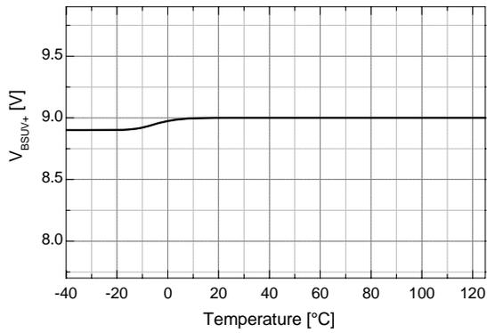
Figure 20. V<sub>BS</sub> UVLO+ vs. Temperature
