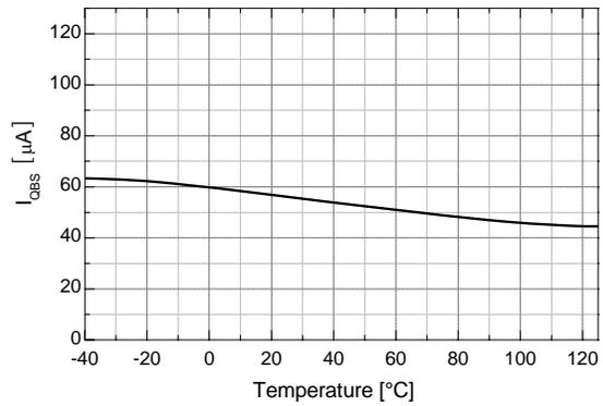
**Figure 15. Quiescent  $V_{BS}$  Supply Current vs. Temperature**
