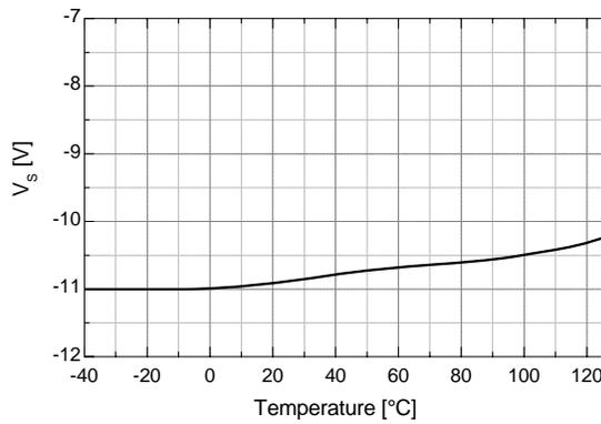
Figure 26. Allowable Negative VS Voltage vs. Temperature
