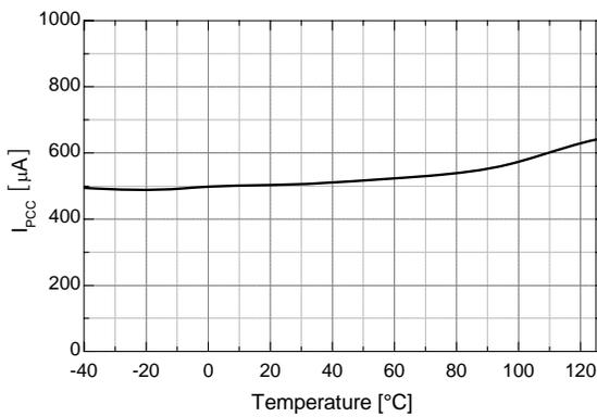
**Figure 16. Operating  $V_{CC}$  Supply Current vs. Temperature**
