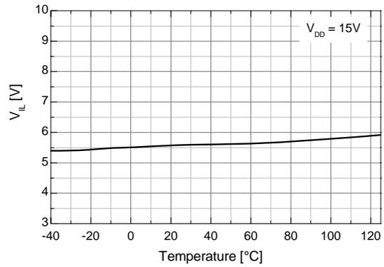
Figure 25. Logic Low Input Voltage vs. Temperature
