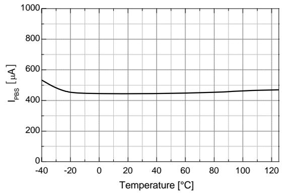
**Figure 17. Operating  $V_{BS}$  Supply Current vs. Temperature**
