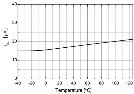
**Figure 13. Logic Input High Bias Current vs. Temperature**
