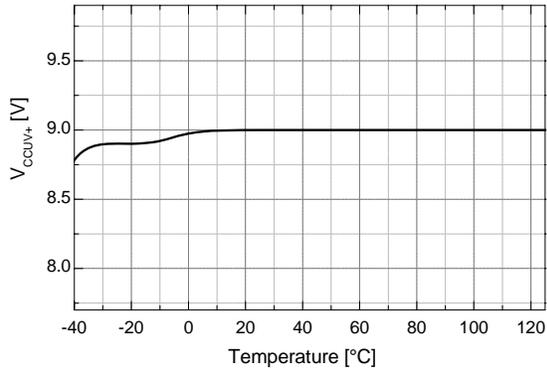
Figure 18. V<sub>CC</sub> UVLO+ vs. Temperature
