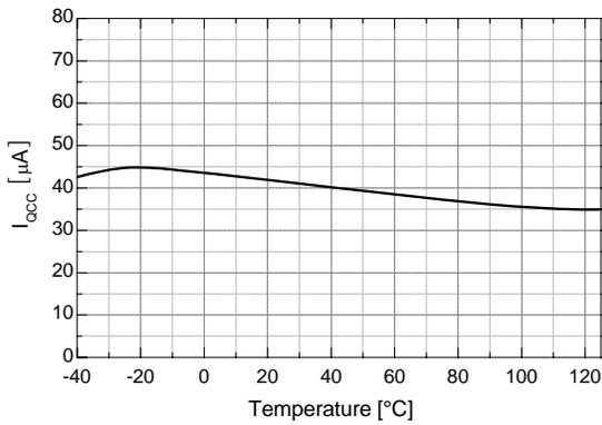
**Figure 14. Quiescent  $V_{CC}$  Supply Current vs. Temperature**
