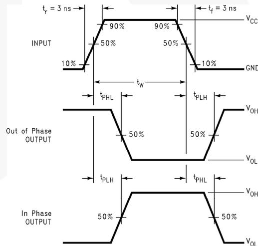
Figure 5. AC Waveforms
