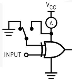
Figure 6. I<sub>CCD</sub> Test Circuit
