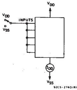
Fig. 11 - Quiescent device current test circuit.
