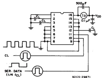
Fig. 10 — Dynamic power dissipation test circuit.
