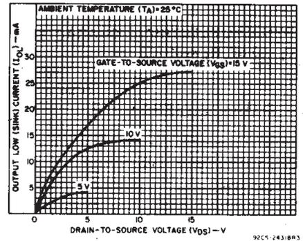
Fig. 3 - Typical output low (sink) current characteristics.
