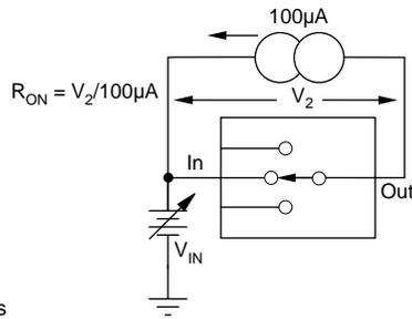
ON RESISTANCE vs ANALOG INPUT VOLTAGE
