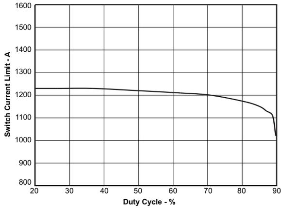
Figure 3. Switch Current Limit vs Duty Cycle
