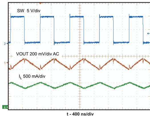
Figure 5. Switching Waveform
