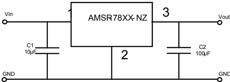
**C1:** A low ESR capacitor is required to keep the noise of the converter to a minimum. Ceramic capacitors are recommended, but tantalum or electrolytic may be used. Typical value is 10µF / 50V.
