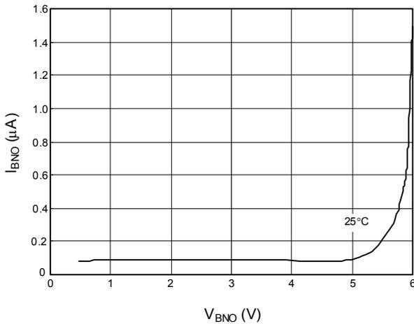
Fig. 13 V<sub>BNO</sub> vs. I<sub>BNO</sub>
