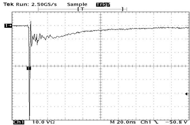
Figure 2. IEC61000-4-2 -8 KV Contact Clamping Voltage
