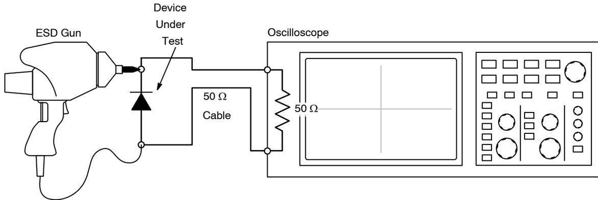
Figure 4. Diagram of ESD Clamping Voltage Test Setup
