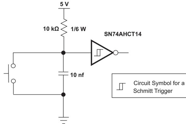
Figure 3. Switch De-bouncer Using Schmitt Trigger Inverter
