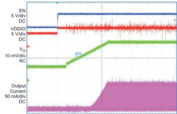
Figure 12. Start-Up Waveform
