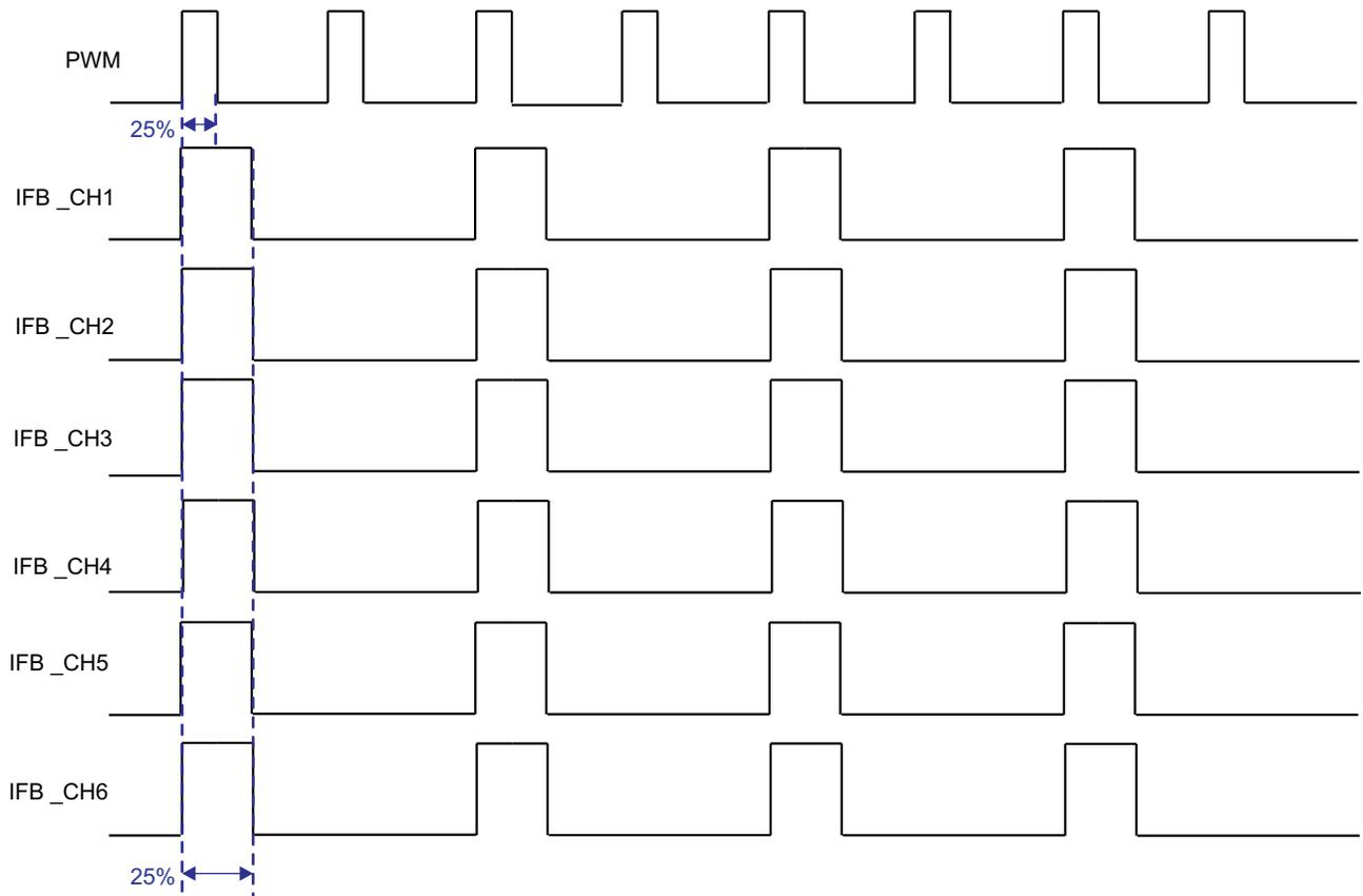
Figure 16. Programmable PWM Dimming Timing Diagram
