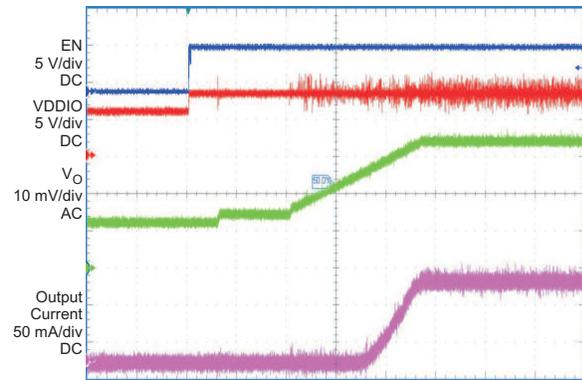
Figure 11. Start-Up Waveform
