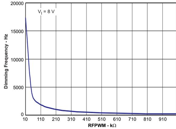
Figure 4. Programmable Dimming
