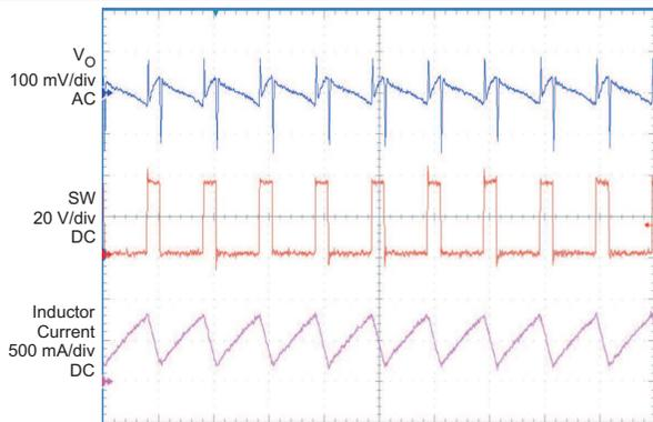
Figure 5. Switch Waveform
