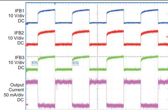
Figure 8. Programmable PWM Waveform
