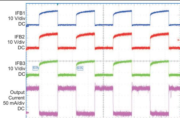
Figure 7. Programmable PWM Waveform
