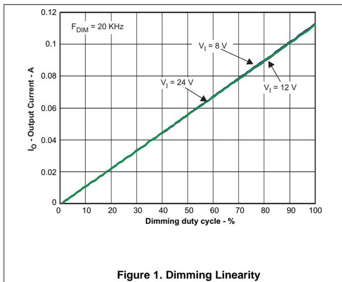
**Figure 1. Dimming Linearity**
