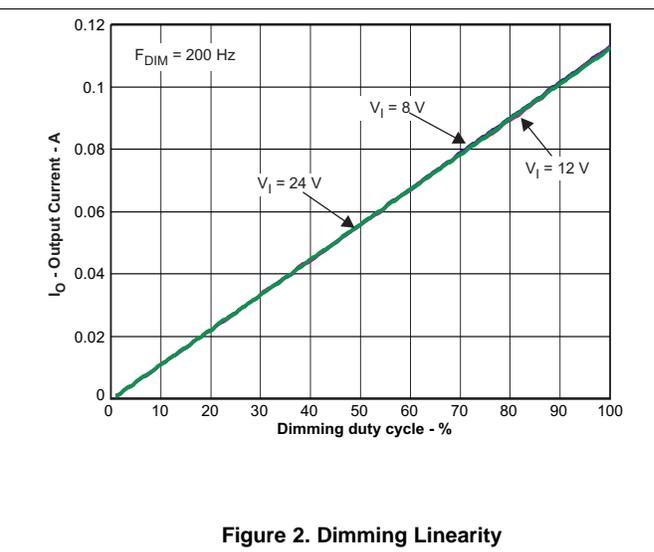
**Figure 2. Dimming Linearity**
