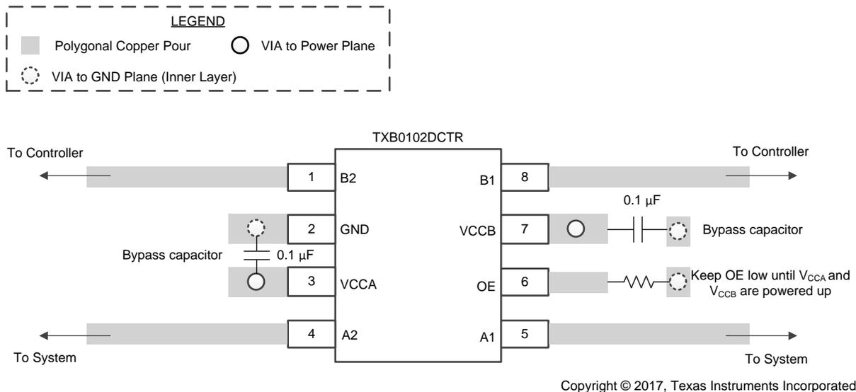
Figure 9. TXB0102 Layout Example
