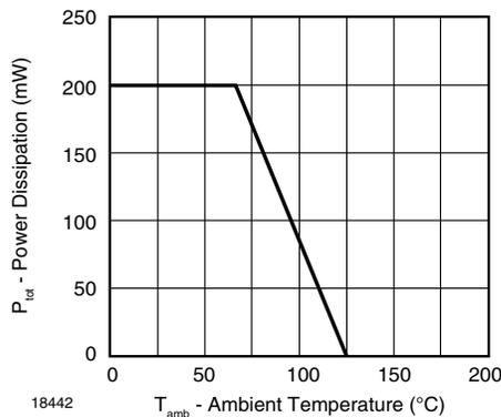
Fig. 1 - Admissible Power Dissipation vs. Ambient Temperature
