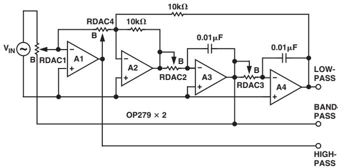
Figure 10. Programmable State Variable Active Filter
