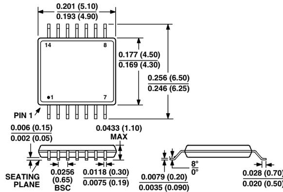
CONTROLLING DIMENSIONS ARE IN MILLIMETERS, INCH DIMENSIONS ARE ROUNDED-OFF MILLIMETER EQUIVALENTS FOR REFERENCE ONLY AND ARE NOT APPROPRIATE FOR USE IN DESIGN
