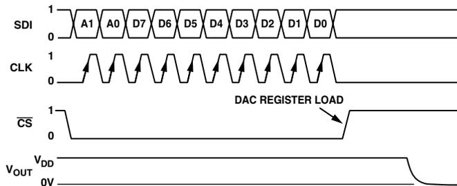
Figure 2a. Timing Diagram
