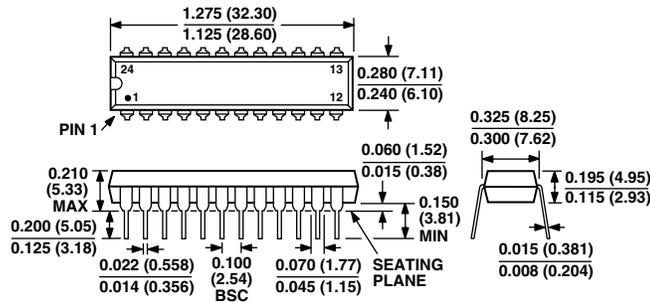
CONTROLLING DIMENSIONS ARE IN MILLIMETERS, INCH DIMENSIONS ARE ROUNDED-OFF MILLIMETER EQUIVALENTS FOR REFERENCE ONLY AND ARE NOT APPROPRIATE FOR USE IN DESIGN
