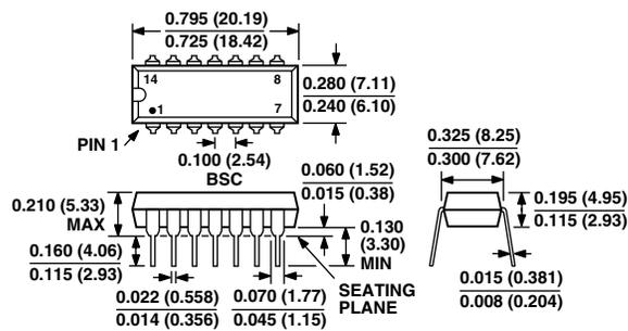
CONTROLLING DIMENSIONS ARE IN MILLIMETERS, INCH DIMENSIONS ARE ROUNDED-OFF MILLIMETER EQUIVALENTS FOR REFERENCE ONLY AND ARE NOT APPROPRIATE FOR USE IN DESIGN
