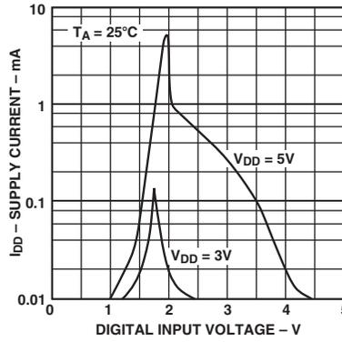
TPC 20. Supply Current vs. Digital Input Voltage
