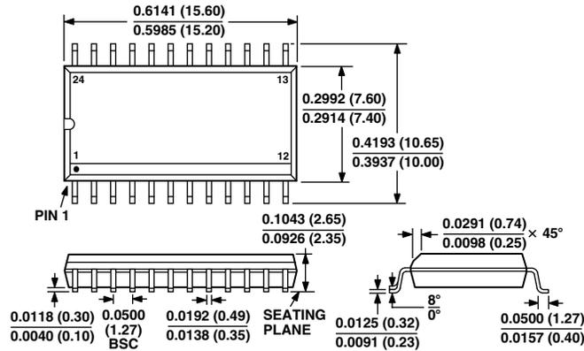
CONTROLLING DIMENSIONS ARE IN MILLIMETERS, INCH DIMENSIONS ARE ROUNDED-OFF MILLIMETER EQUIVALENTS FOR REFERENCE ONLY AND ARE NOT APPROPRIATE FOR USE IN DESIGN
