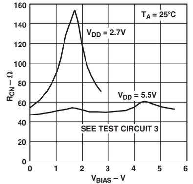
TPC 24. AD8403 Incremental Wiper ON Resistance vs. V<sub>DD</sub>
