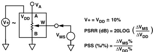
Test Circuit 4. Power Supply Sensitivity (PSS, PSRR)
