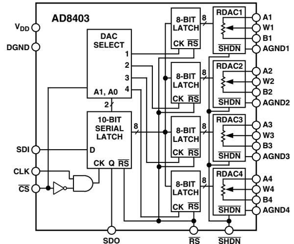
to an end-to-end open circuit condition on the A terminal and shorts the wiper to the B terminal, achieving a microwatt power shutdown state. When  $\overline{SHDN}$  is returned to logic high, the previous latch settings put the wiper in the same resistance setting prior to shutdown. The digital interface is still active in shutdown so that code changes can be made that will produce new wiper positions when the device is taken out of shutdown.
