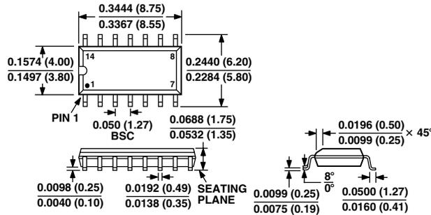
CONTROLLING DIMENSIONS ARE IN MILLIMETERS, INCH DIMENSIONS ARE ROUNDED-OFF MILLIMETER EQUIVALENTS FOR REFERENCE ONLY AND ARE NOT APPROPRIATE FOR USE IN DESIGN
