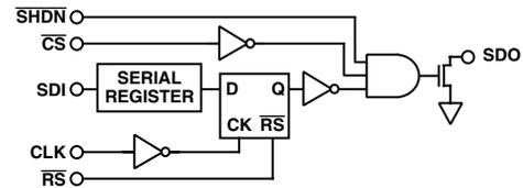
Figure 6. Detail SDO Output Schematic of the AD8403
