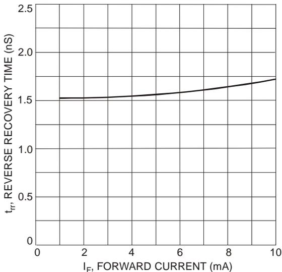
Figure 5 Reverse Recovery Time vs. Forward Current
