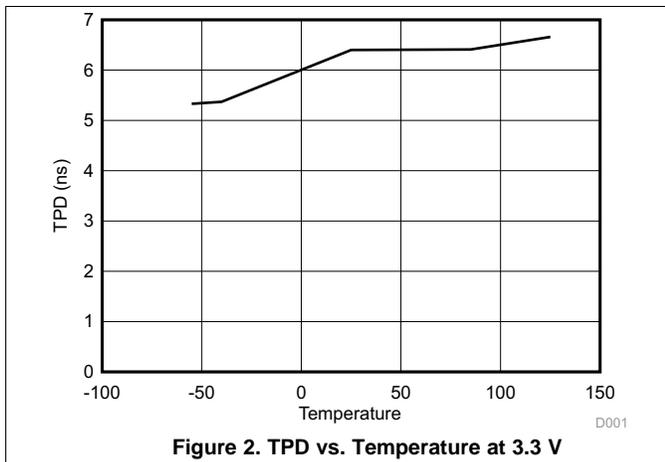
Figure 2. TPD vs. Temperature at 3.3 V
