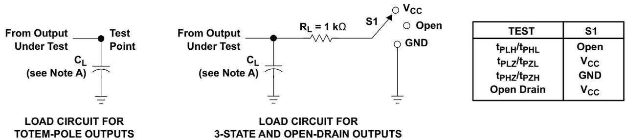
LOAD CIRCUIT FOR TOTEM-POLE OUTPUTS
