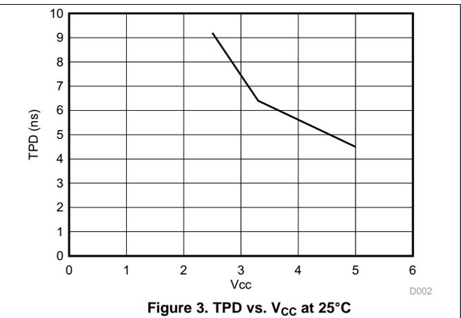
Figure 3. TPD vs. V<sub>CC</sub> at 25°C
