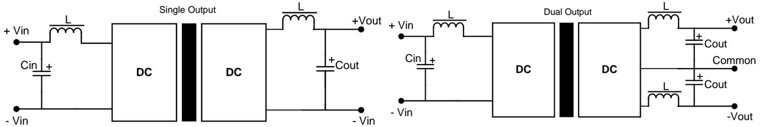
If it is required to decrease the input/output ripple an “LC” filter network can be installed on the input and output of the converter (see above).
