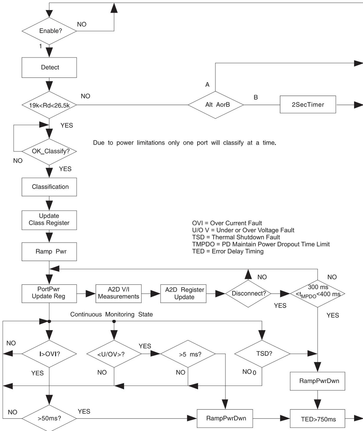
Figure 7. The Basic Flow for Auto Mode
