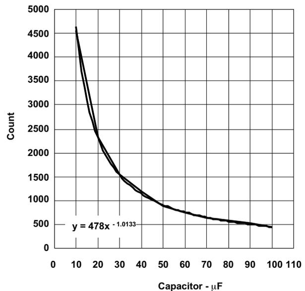
Figure 19. A/D Counts vs Legacy Port Capacitance
