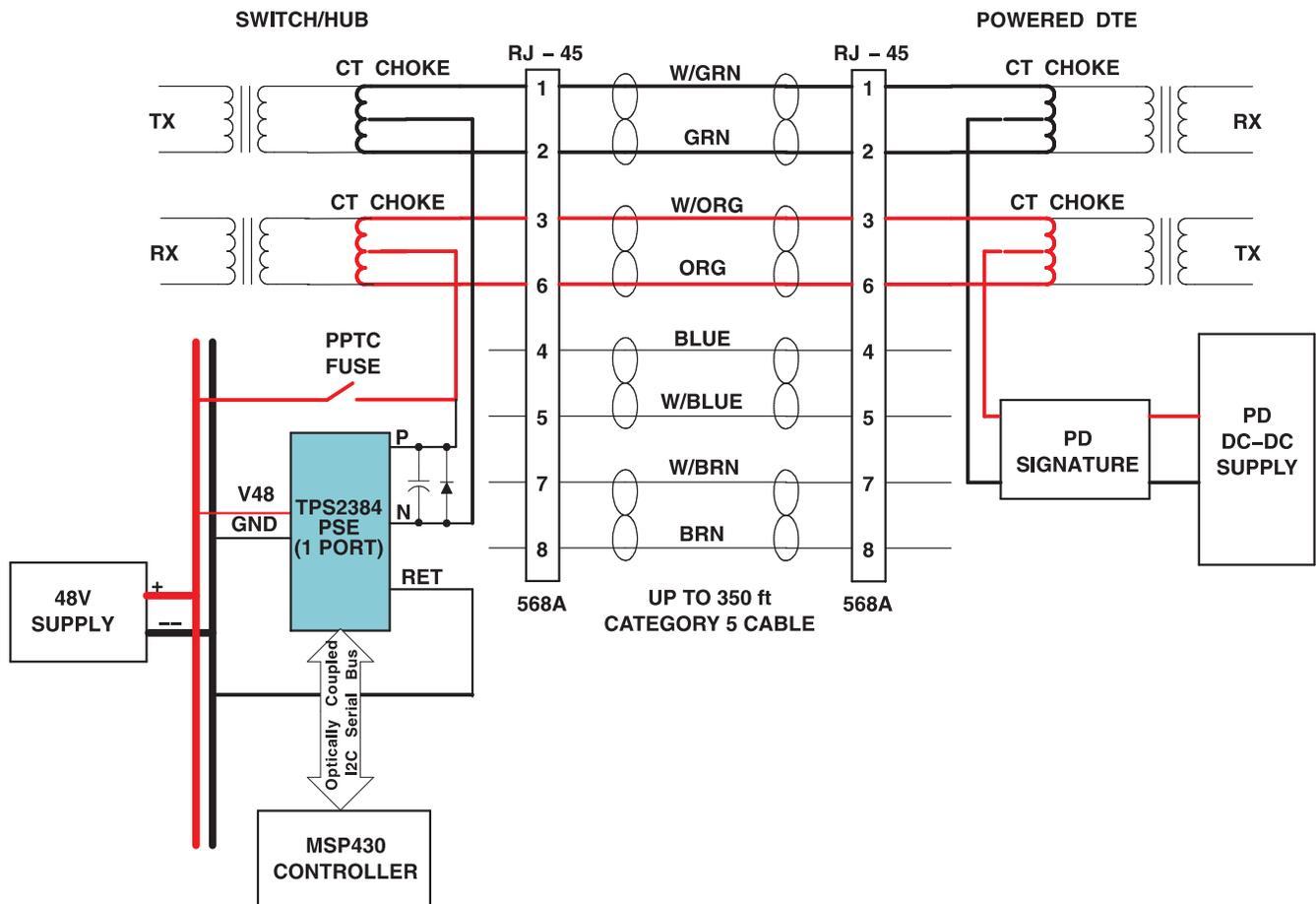
NOTE: A fuse may be required to provide additional protection if isolation is lost or the low-side current sense fails.
