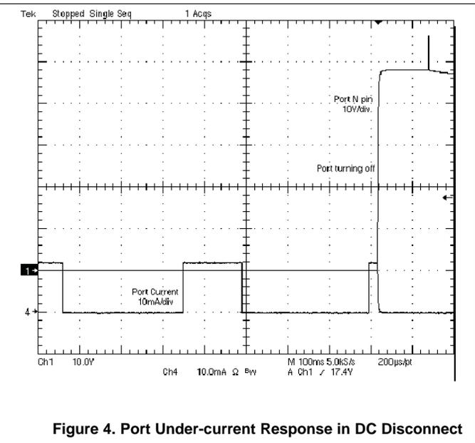
**Figure 4. Port Under-current Response in DC Disconnect**
