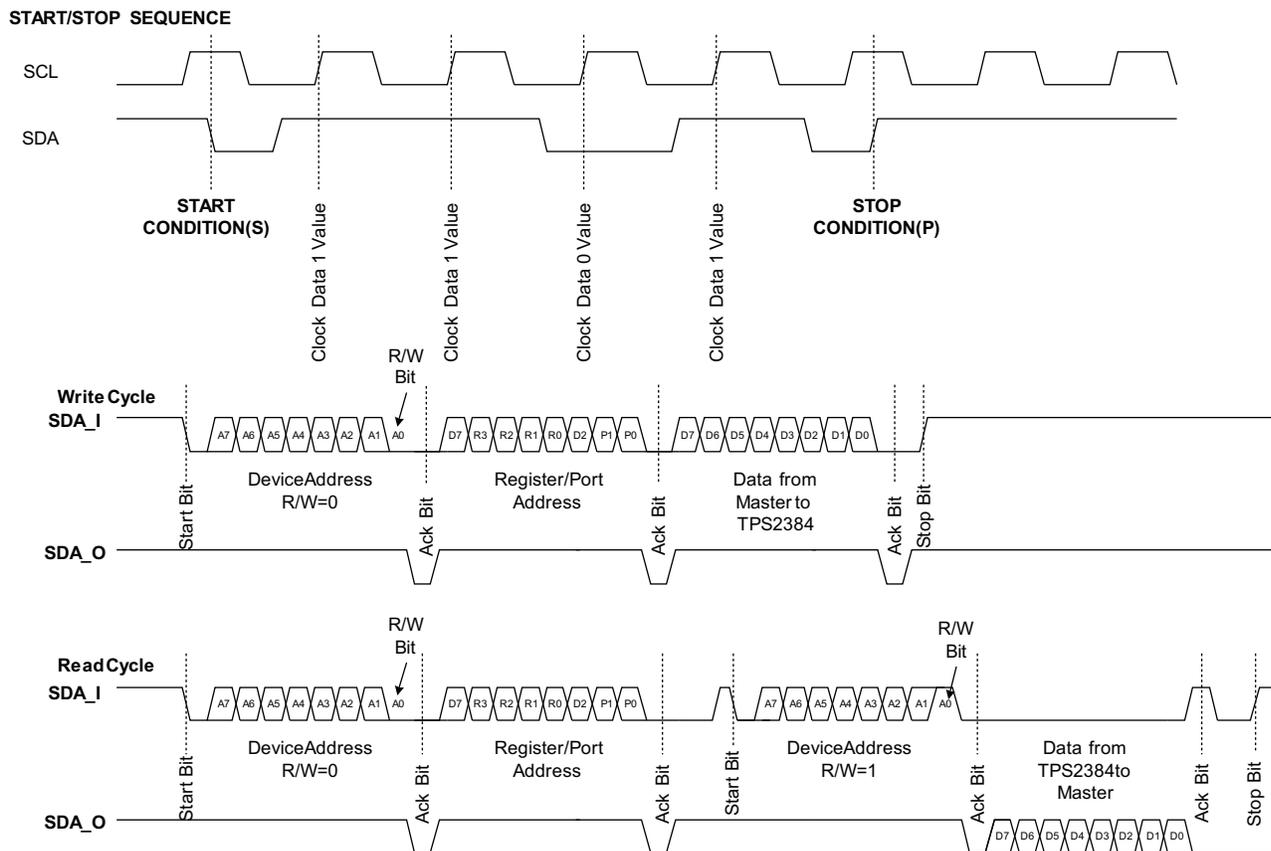
Figure 22. I<sup>2</sup>C Read/Write Cycles
