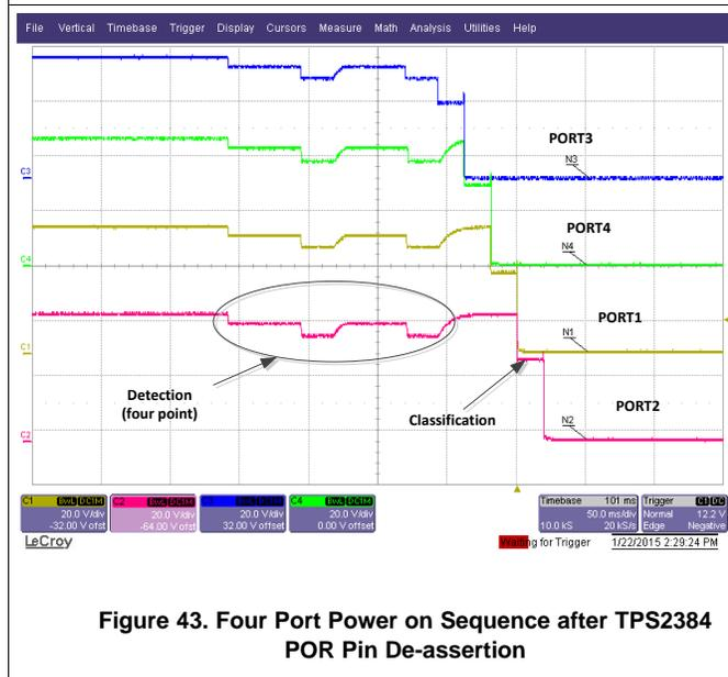
Figure 43. Four Port Power on Sequence after TPS2384 POR Pin De-assertion
