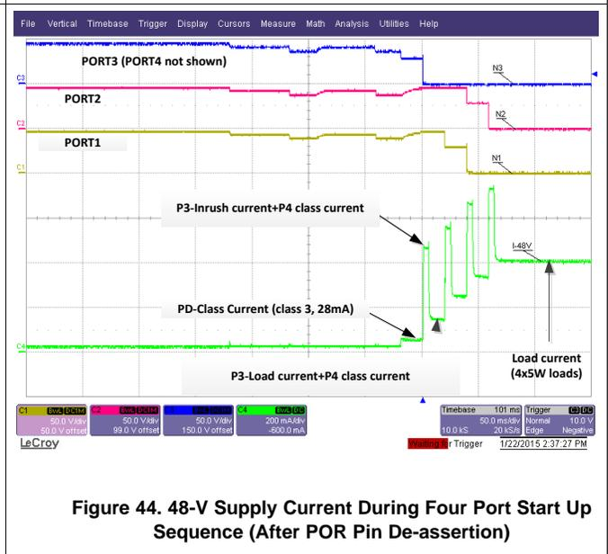
Figure 44. 48-V Supply Current During Four Port Start Up Sequence (After POR Pin De-assertion)
