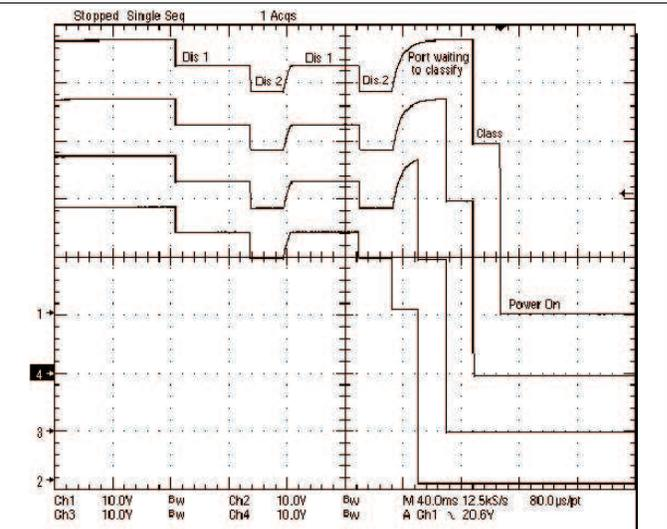
**Figure 2. Four Port Discovery, Class, Power On**
