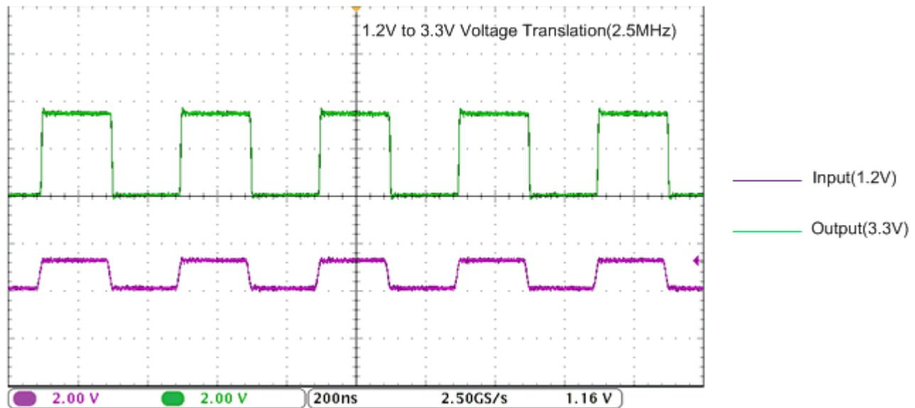
Figure 6. Translation Up (1.2 V to 3.3 V) at 2.5 MHz
