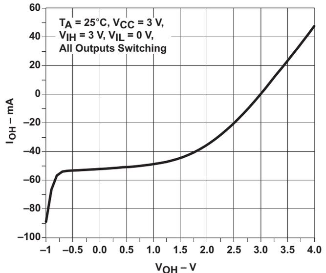
Figure 6. Output Drive Current (I<sub>OH</sub>) vs HIGH-level Output Voltage (V<sub>OH</sub>)
