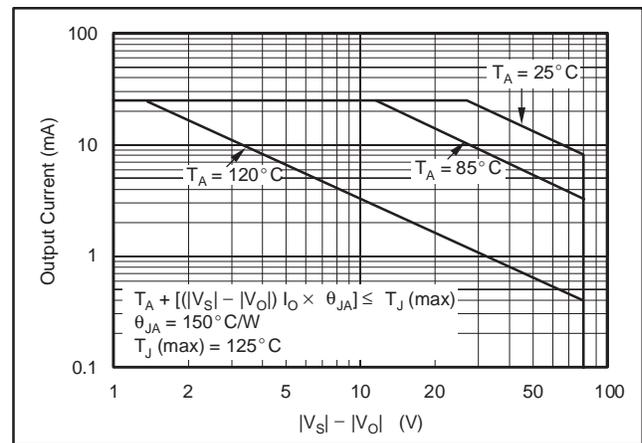
Figure 8. SO-8 (non PowerPAD) Safe Operating Area
