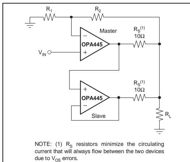
Figure 4. Parallel Amplifiers Increase Output Current Capability
