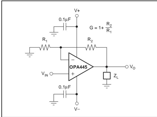
Figure 1. The OPA445 Configured as a Noninverting Amplifier
