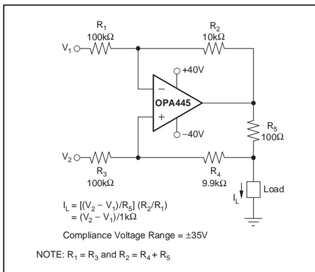
Figure 15. Voltage-to-Current Converter
