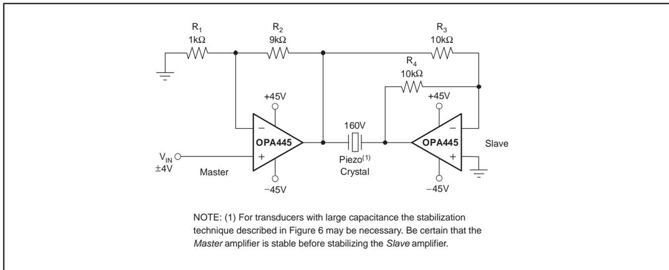
Figure 17. Bridge Circuit Doubles Voltage for Piezo Crystals
