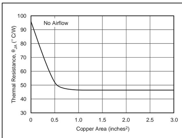
Figure 12. Thermal Resistance vs Circuit Board Copper Area
