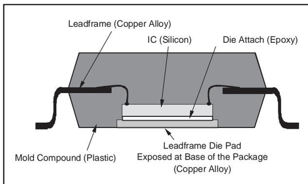
Figure 13. Section View of a PowerPAD Package
