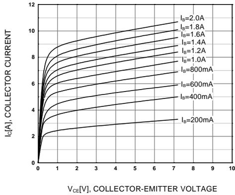
Figure 1. Static Characteristic
