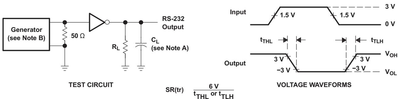
A.  $C_L$  includes probe and jig capacitance
