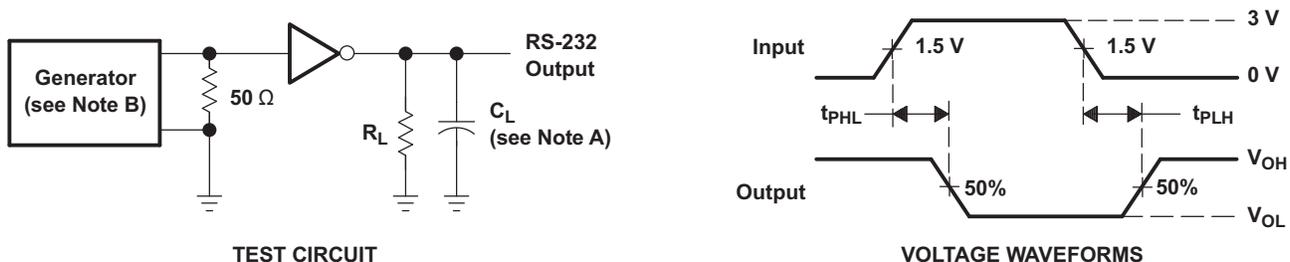
A.  $C_L$  includes probe and jig capacitance
