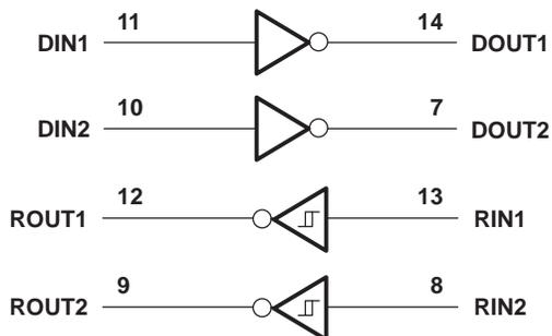
**Figure 6. Logic Diagram**
