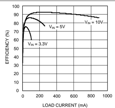
Figure 12. Efficiency vs Load Current ( $V_{OUT} = 15\text{ V}$ ) - "X"
