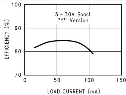
**Figure 33. Efficiency vs. Load Current (5 - 30V Y-version)**
