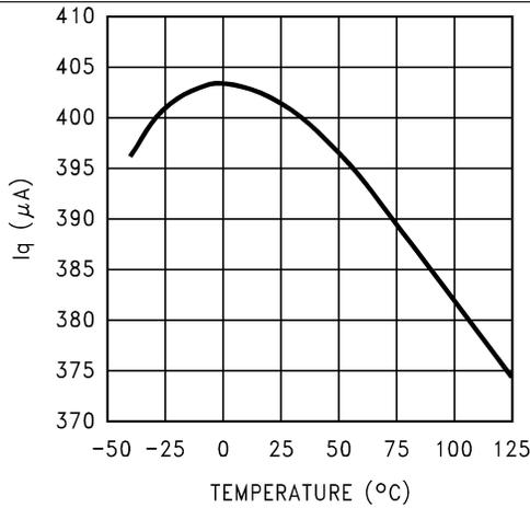
Figure 1.  $I_q V_{IN}$  (Active) vs Temperature - "X"
