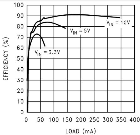
Figure 21. Efficiency vs Load ( $V_{OUT} = 30\text{ V}$ ) - "Y"
