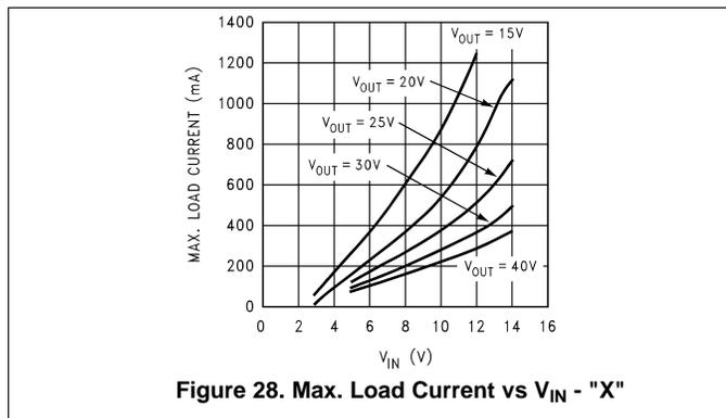
**Figure 28. Max. Load Current vs V\_IN - "X"**
