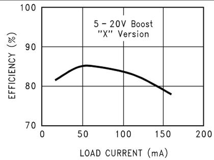
**Figure 32. Efficiency vs. Load Current (5-20V X-version)**
