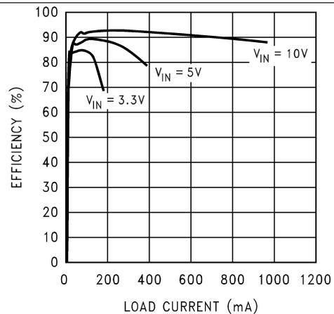
Figure 18. Efficiency vs Load ( $V_{OUT} = 15\text{ V}$ ) - "Y"
