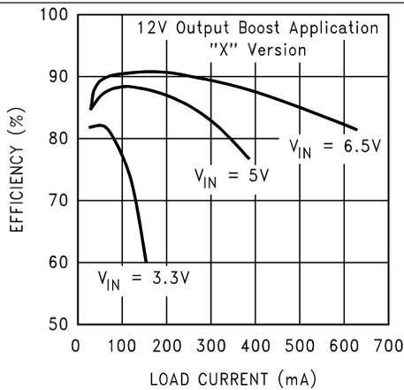
Figure 11. Efficiency vs Load Current ( $V_{OUT} = 12\text{ V}$ ) - "X"
