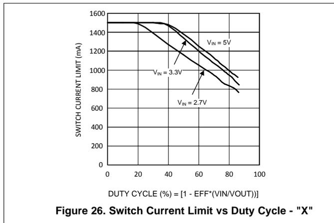
**Figure 26. Switch Current Limit vs Duty Cycle - "X"**
