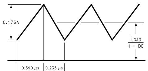
**Figure 25. 10-μH Inductor Current, 5-V – 12-V Boost (LM2733X)**
