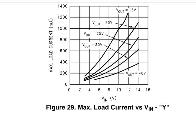
**Figure 29. Max. Load Current vs V\_IN - "Y"**
