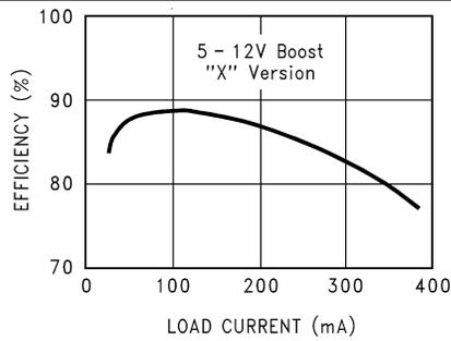
**Figure 31. Efficiency vs. Load Current (5-12V, X-version)**
