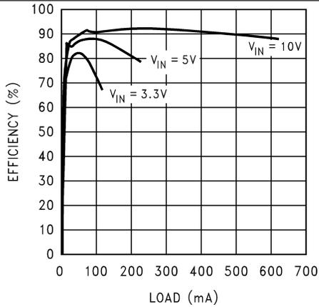
Figure 19. Efficiency vs Load ( $V_{OUT} = 20\text{ V}$ ) - "Y"
