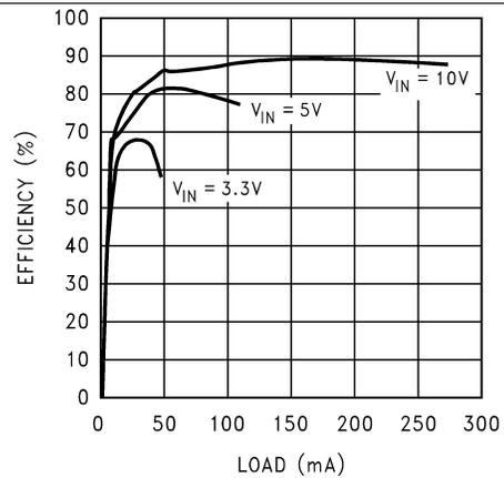
Figure 22. Efficiency vs Load ( $V_{OUT} = 35\text{ V}$ ) - "Y"
