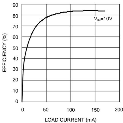
Figure 17. Efficiency vs Load Current ( $V_{OUT} = 40\text{ V}$ ) - "X"
