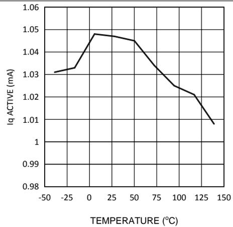
Figure 2.  $I_q V_{IN}$  (Active) vs Temperature - "Y"
