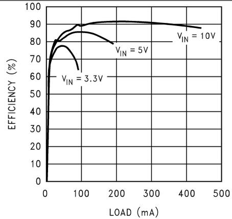
Figure 20. Efficiency vs Load ( $V_{OUT} = 25\text{ V}$ ) - "Y"
