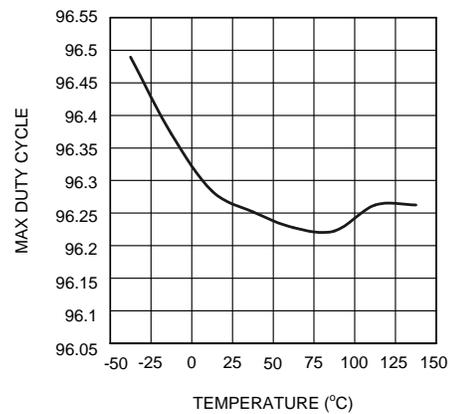
Figure 6. Max. Duty Cycle vs Temperature - "Y"
