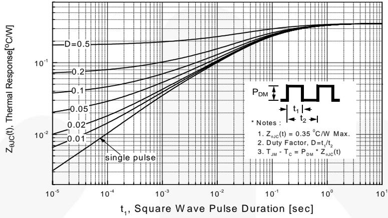
**Figure 11-2. Transient Thermal Response Curve - FDPF52N20T**
