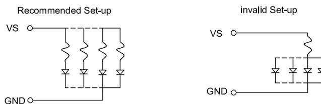
3. The driving circuit should be designed to protect the LED against reverse voltages and transient voltage spikes when the circuit is powered up or shut down.
