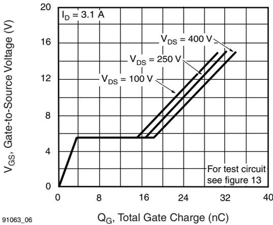
Fig. 6 - Typical Gate Charge vs. Drain-to-Source Voltage
