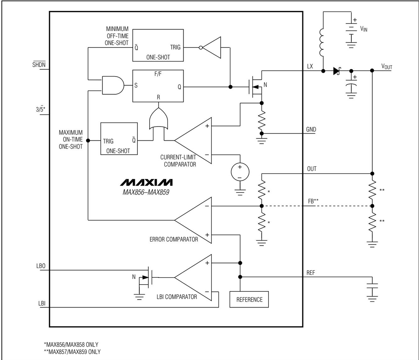
Figure 1. Block Diagram
