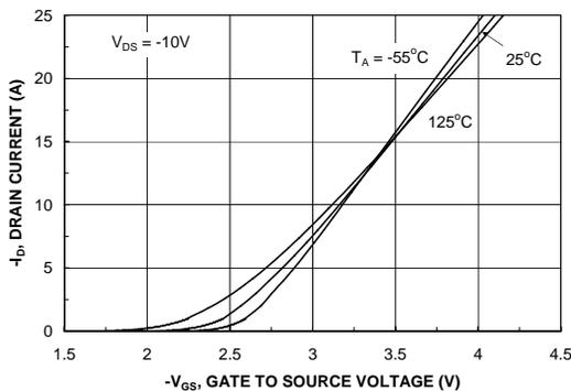
**Figure 17. Transfer Characteristics.**
