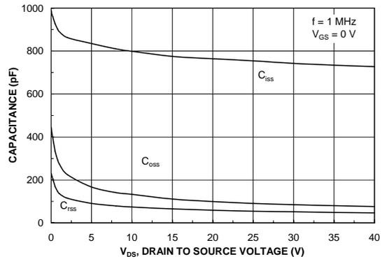
Figure 8. Capacitance Characteristics.
