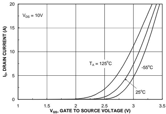
Figure 5. Transfer Characteristics.
