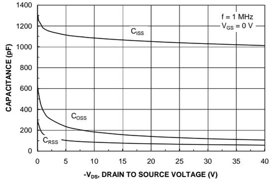
**Figure 20. Capacitance Characteristics.**
