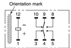
Note: Check carefully the coil polarity of the Relay.
