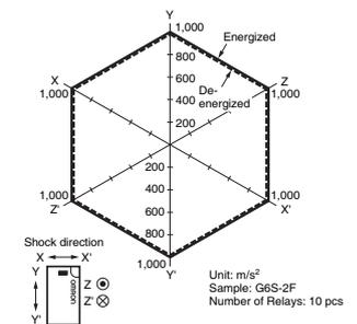
Conditions: Shock is applied in ±X, ±Y, and ±Z directions three times each with and without energizing the Relays to check the number of contact malfunctions.
