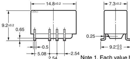
Note 1. Each value has a tolerance of  $\pm 0.3$  mm.
