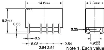
Note 1. Each value has a tolerance of ±0.3 mm.
