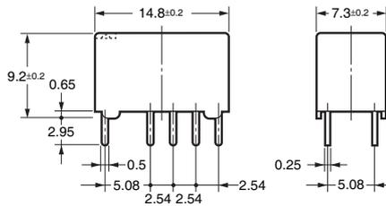
Note: Each value has a tolerance of ±0.3 mm.
