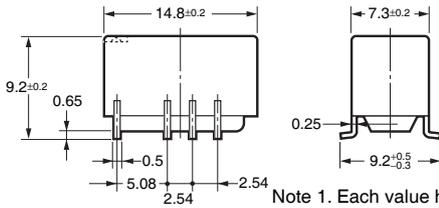
Note 1. Each value has a tolerance of  $\pm 0.3$  mm.
