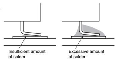
Visually check that the Relay is properly soldered.
