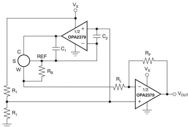
**Figure 1. OPA2379 in Portable Gas Meter Application**
