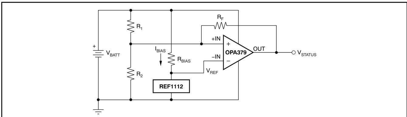
Figure 23. Battery Monitor
