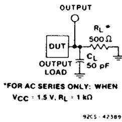
\*FOR AC SERIES ONLY: WHEN  $V_{CC} = 1.5$  V,  $R_L = 1$  k $\Omega$
