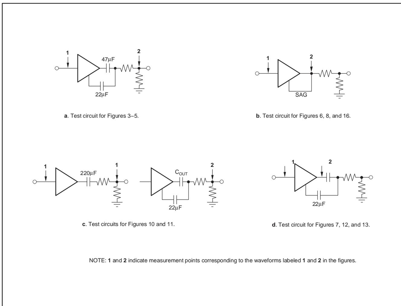
**Figure 2. Test Circuits Used for Figures 3–13**
