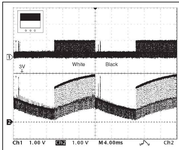
**Figure 7. Output Swing with 33μF on 3V Supply**
