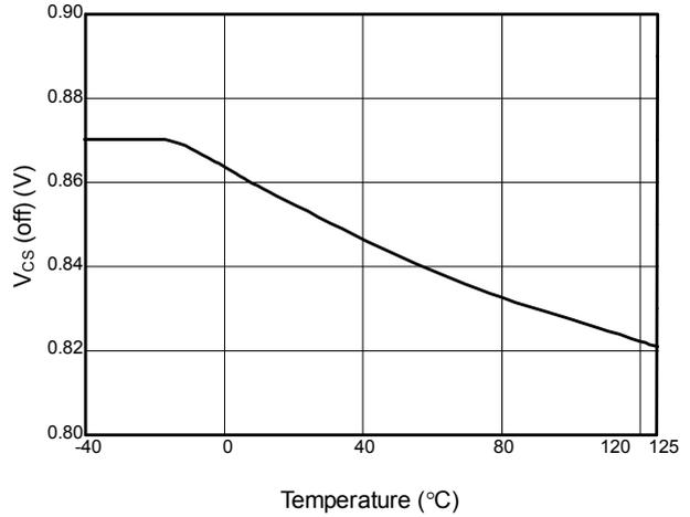
Fig. 8 V<sub>CS</sub> (off) vs. Temperature
