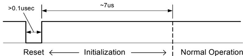
Figure 7 Reset timing
