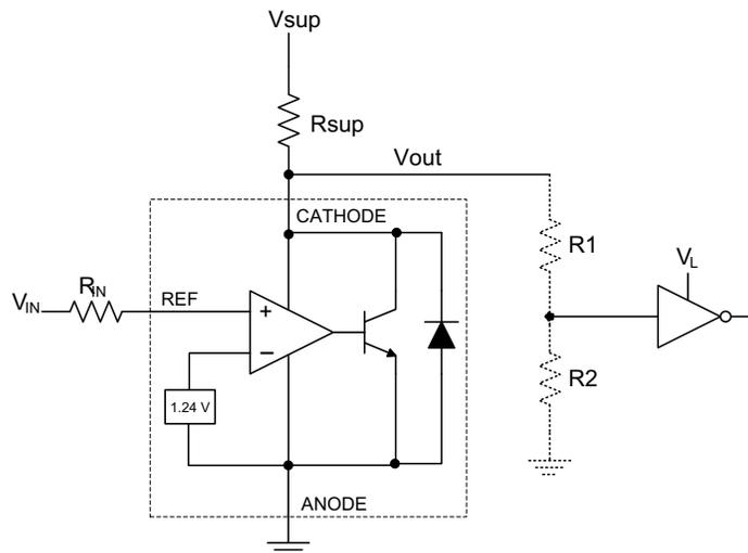
**Figure 26. Comparator Application Schematic**
