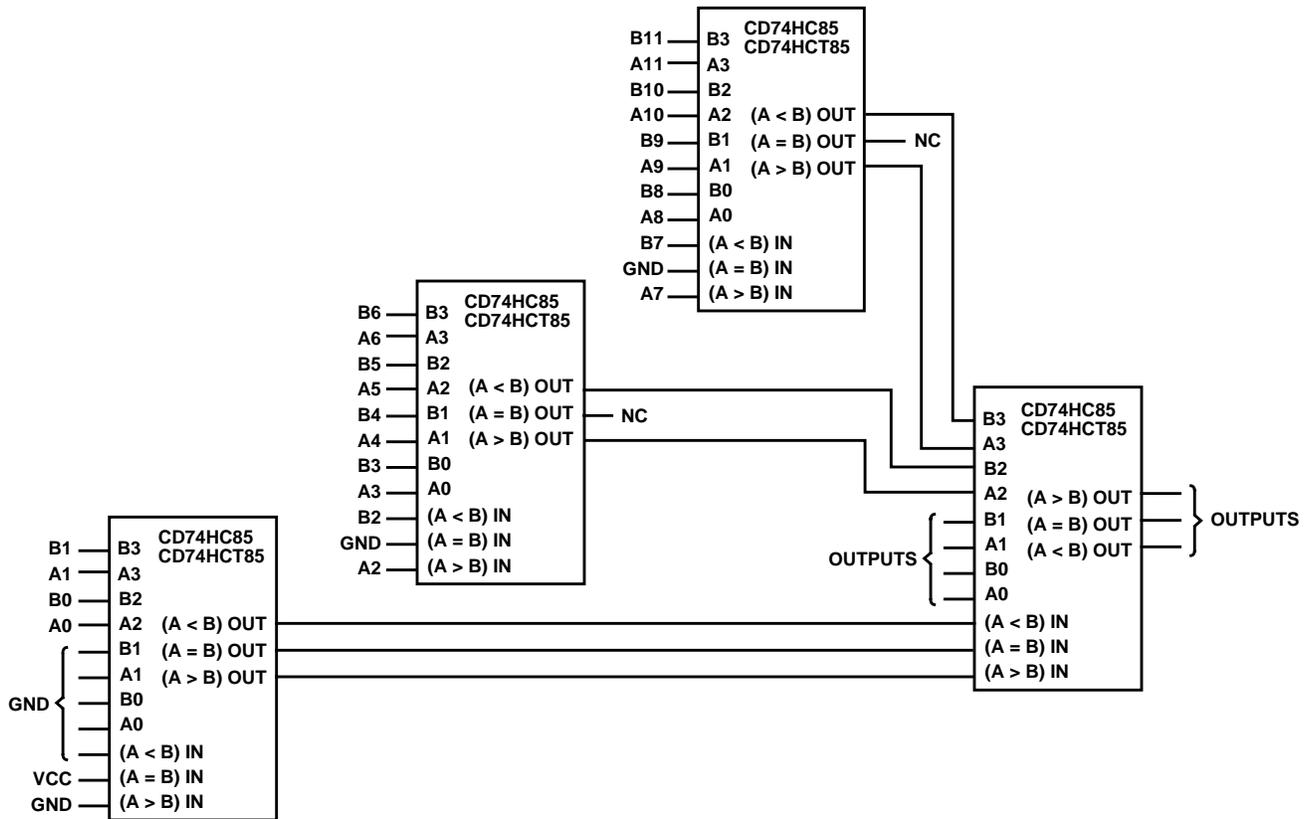
FIGURE 4. PARALLEL CASCADING - COMPARING 12-BIT WORDS
