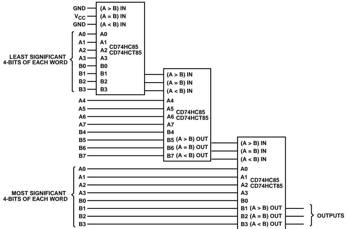
FIGURE 3. SERIES CASCADING - COMPARING 12-BIT WORDS
