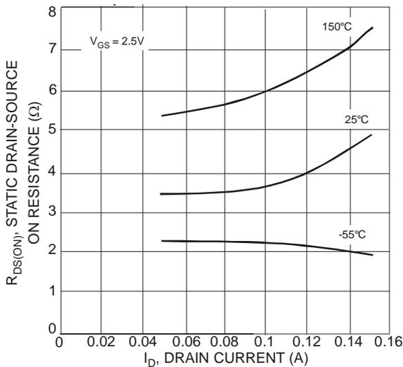
Fig. 5 Drain-Source On Resistance vs. Drain Current
