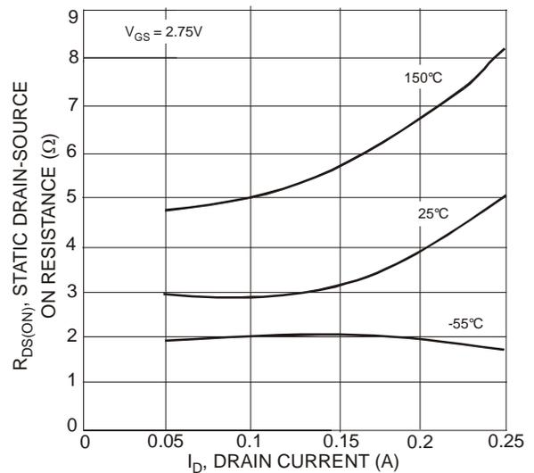
Fig. 6 Drain-Source On Resistance vs. Drain Current
