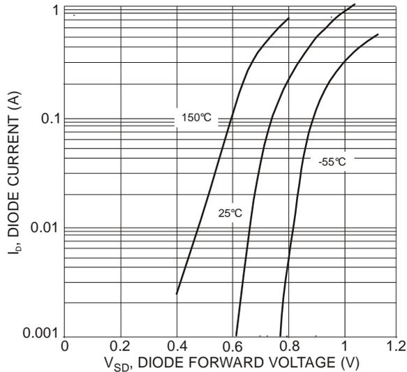
Fig. 9 Body Diode Current vs. Body Diode Voltage
