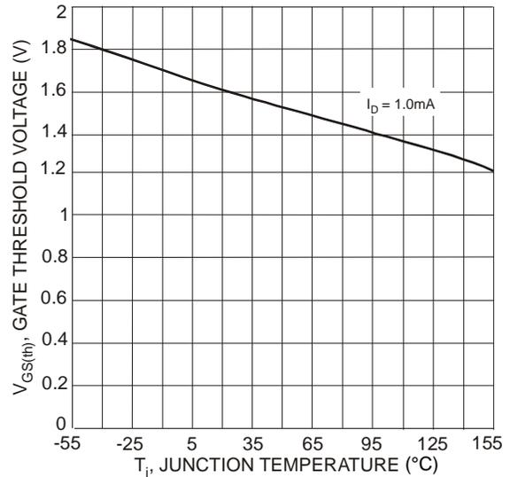
Fig. 4 Gate Threshold Voltage vs. Junction Temperature
