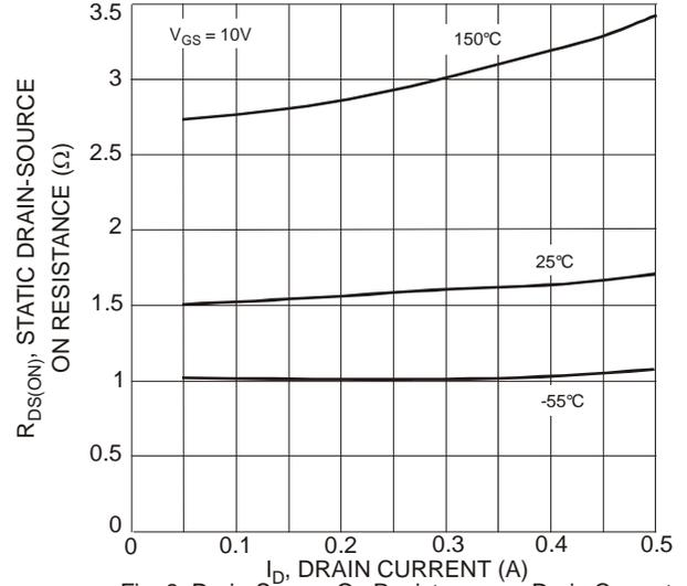
Fig. 8 Drain-Source On Resistance vs. Drain Current
