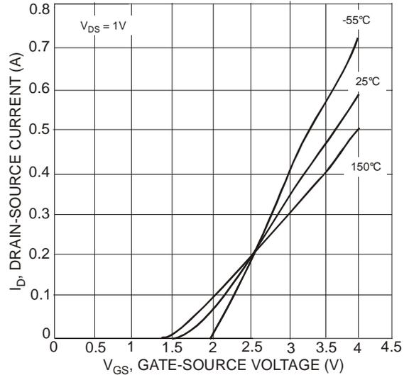
Fig. 2 Transfer Characteristics
