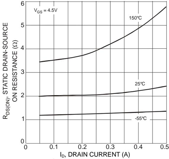
Fig. 7 Drain-Source On Resistance vs. Drain Current
