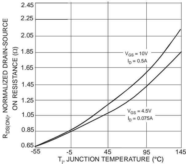
Fig. 3 Drain-Source On Resistance vs. Junction Temperature
