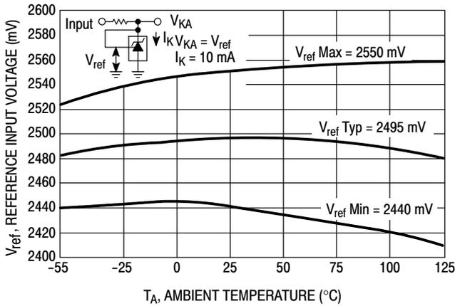
Figure 6. Reference Input Voltage versus Ambient Temperature
