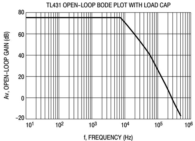
Figure 33. Example 2 Circuit Open Loop Gain Plot
