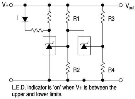
L.E.D. indicator is 'on' when V+ is between the upper and lower limits.
