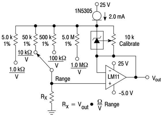
Figure 28. Linear Ohmmeter
