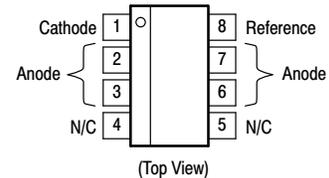
This is an internally modified SOIC-8 package. Pins 2, 3, 6 and 7 are electrically common to the die attach flag. This internal lead frame modification increases power dissipation capability when appropriately mounted on a printed circuit board. This modified package conforms to all external dimensions of the standard SOIC-8 package.
