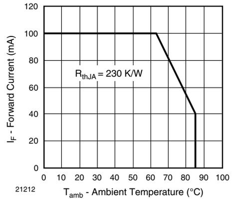
Fig. 2 - Forward Current Limit vs. Ambient Temperature
