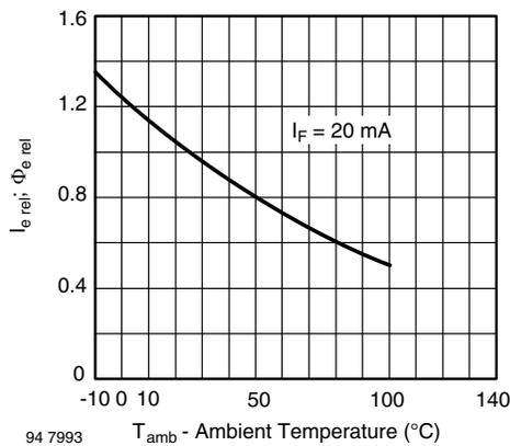
Fig. 7 - Rel. Radiant Intensity/Power vs. Ambient Temperature
