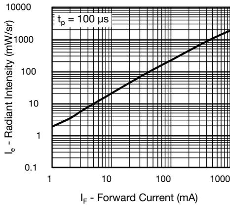
Fig. 5 - Radiant Intensity vs. Forward Current
